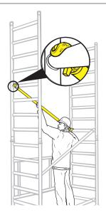
**9** Attach one stabiliser to each corner of the tower. Loosen clamp and place around vertical tube, tighten using handle. Refer to Stabiliser Section for positioning diagrams. To attach one stabiliser to each corner of the tower loosen clamp and place around vertical tube, tighten using handle.
