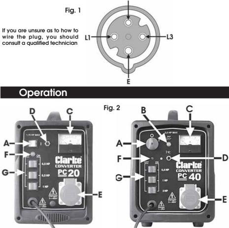
Before inserting the output plug, switch all three switches (G) to OFF. Then switch the converter ON, using the ON/OFF switch (A) on the front panel. In this condition the lamp (B) will illuminate. In the case of the PC20, the rocker switch A will illuminate.
