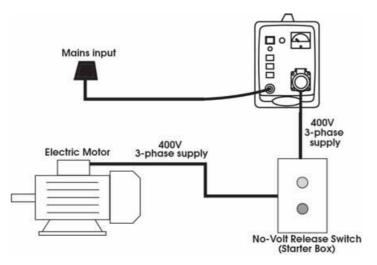
Typical Wiring Diagram for 230V to 400V Phase Converter Standard on-line starting.
